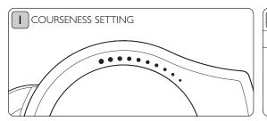
Adjust the degree of grinding by twisting the hopper and aligning the arrow on the hopper with the desired setting.
