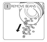
Remove any beans from the hopper by turning it upside down over a bowl or plate.
