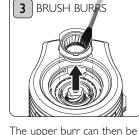
The upper burr can then be removed by lifting it straight up. Use a soft-bristle brush to clean the burrs. Wipe the body clean with a damp cloth.
