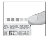
You can find out what the water hardness is by using the Aquadur® test strip supplied as standard.
