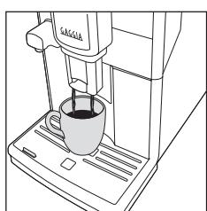
**Note:** to prepare two cups of Espresso or Espresso Lungo, press the button of the preferred beverage twice. The machine performs two consecutive grinding cycles automatically.
