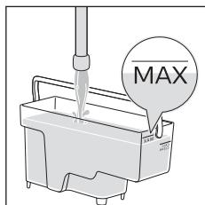
Remove the water tank, rinse it and fill it with running water up to the MAX level. Make sure that the water tank is fully inserted into the compartment.
