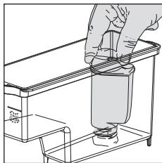
Insert the "INTENZA +" water filter in the empty water tank and push it down to the lowest point.
