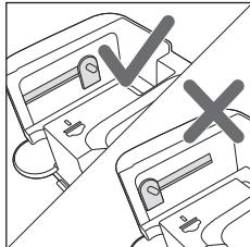
**Note:** before putting the milk dispensing spout back in the upper part of the milk carafe, place the pin inside the upper part in its right position. If the pin is not in its right position, you cannot put the milk dispensing spout back in the upper part of the milk carafe.
