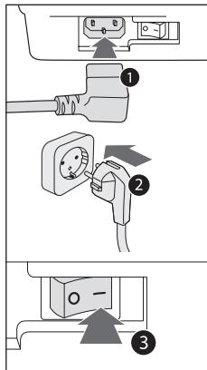
Insert the plug into the socket located on the back of the machine and the other end of the power cord into a wall socket with suitable power voltage.
