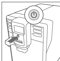
The standby button will blink. Press the button to switch on the machine.
